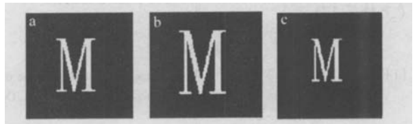
Fig 2 a-undistorted image b- scaled with a factor 1.2 c- scaled with a factor 0.8
